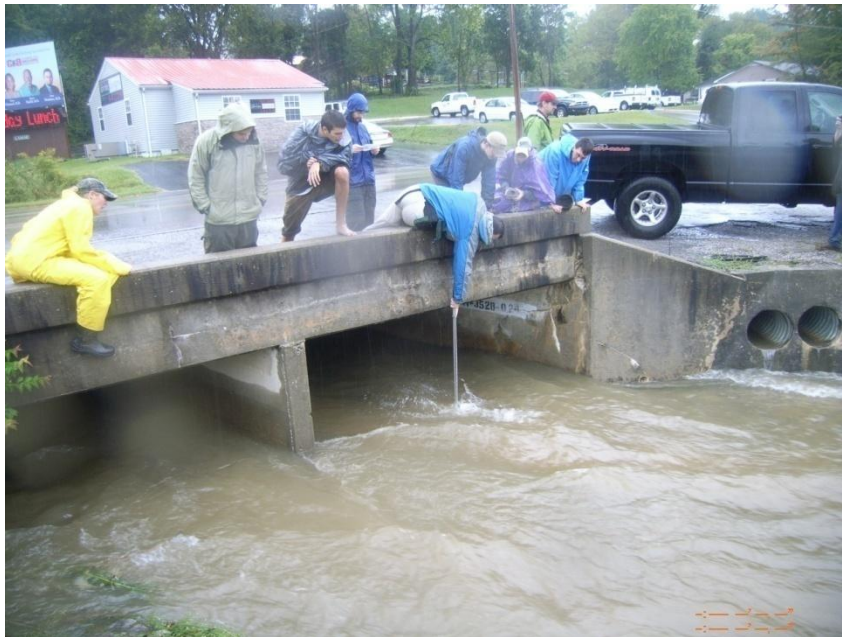
Figure 10. Hydrogeology students making discharge measurement along Short Creek (near intersection of Lowe and Stevens St.) during 9-16-09 storm.
